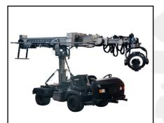
**32' Hydrascope** Fully submersible telescopic crane when used with sliding weights system. Pair with the Amphibian Remote Head for spectacular underwater shots.
