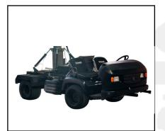
**Raptor** This base offers efficient repositioning of telescopic cranes and fixed cranes with its auto leveling feature. Compatible with the 40', 32', and 20' Hydrascopes, as well as the 23' Scorpio.
