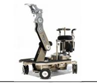
*Pee Wee IV+* Revolutionary three-mode transmission with conventional, crab & round steering modes.
